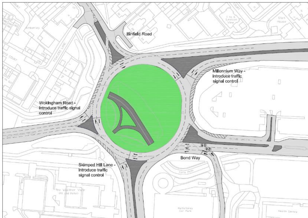
Figure B – Western Roundabout with concept mitigation
