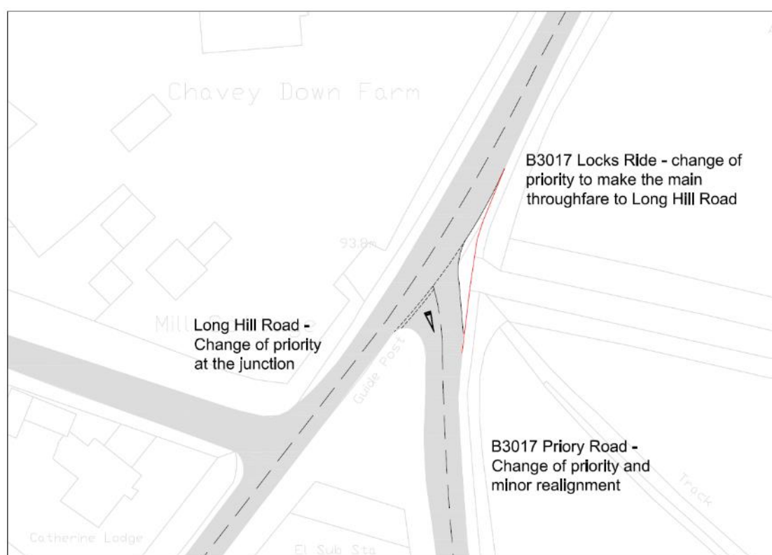
Figure B – B3017 Locks Ride / Long Hill Road with concept mitigation
