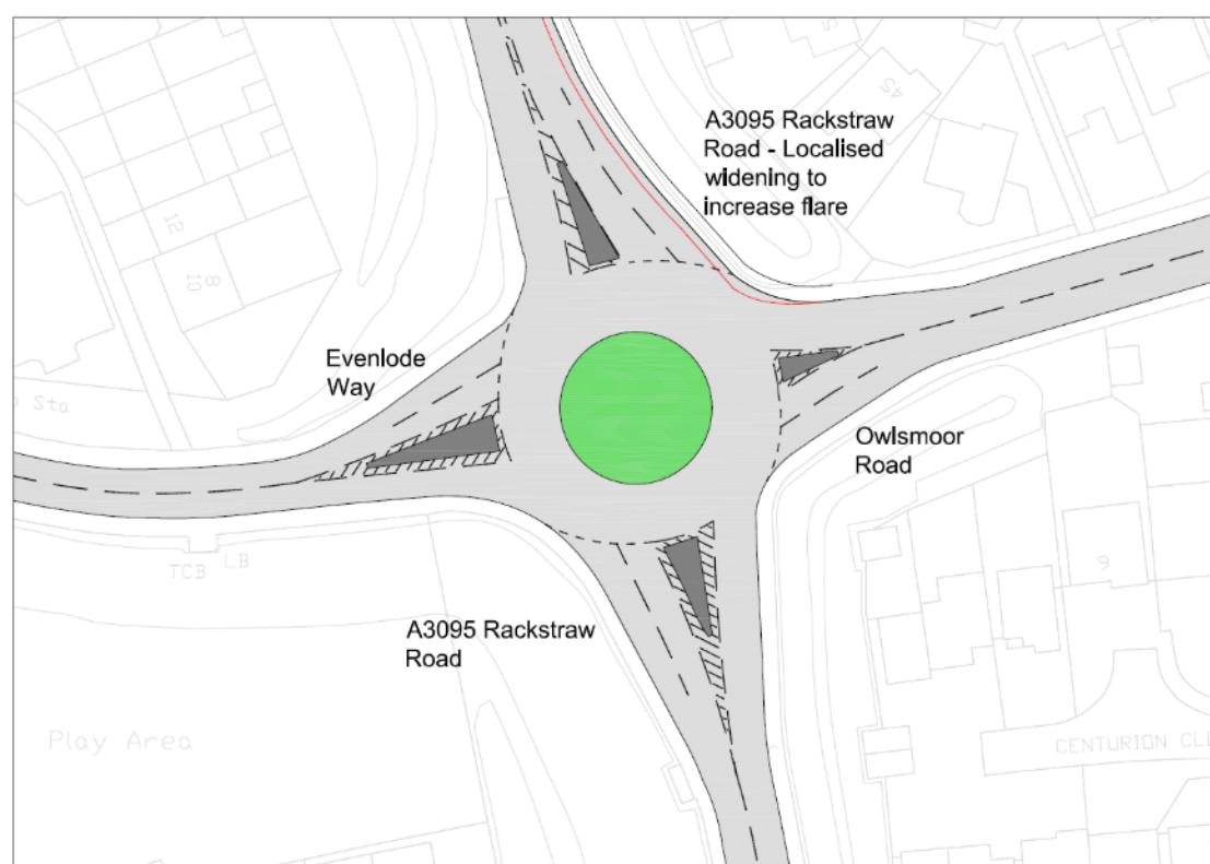
Figure B - Evenlode Way Roundabout with concept mitigation
