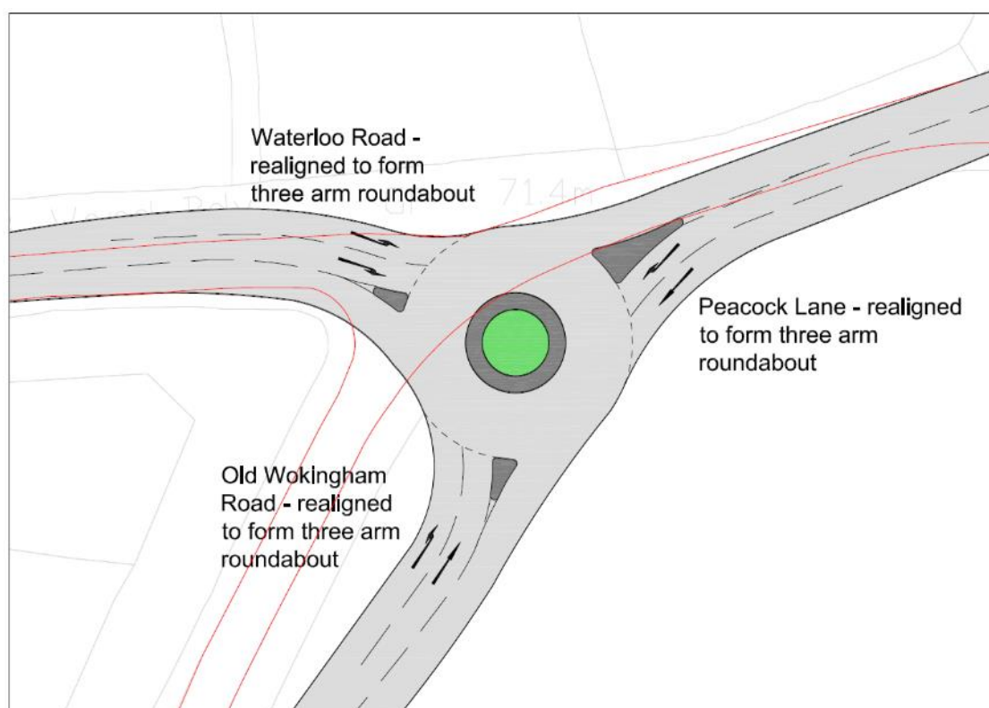
Figure B – Waterloo Road / Old Wokingham Road with concept mitigation
